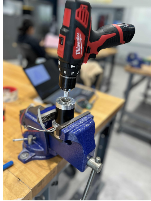
Fig. 14. AC Generator Testing
